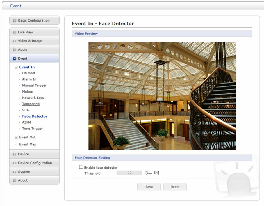
This is used to detect a human face in the scene to trigger event with a bounding box for the detected face. Select “Enable face detector” to activate the Face Detector. Set threshold for detection sensitivity.
