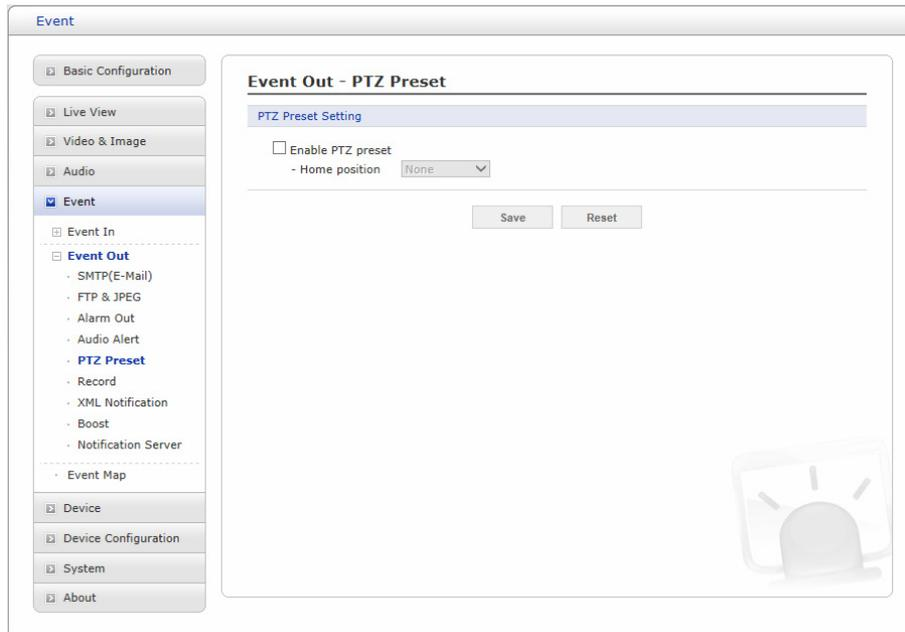
When the camera detects an event, you can move the camera to a predefined preset position. Check the box to enable the service and return to the Home position once the event has ended.
