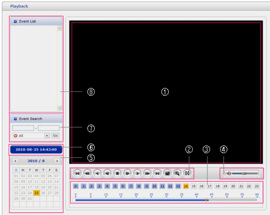
The Playback window contains a list of recordings made to the memory card. It shows each recording's start time, length, the event type used to start the recording, calendar and time slice bar indicates if the recording is existed or not.
