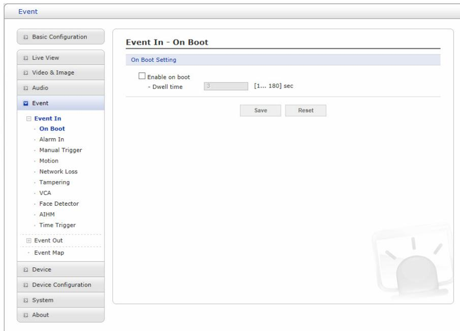
This is used to trigger an event every time the network camera is started. Select “Enable on boot” to activate the On Boot event.
