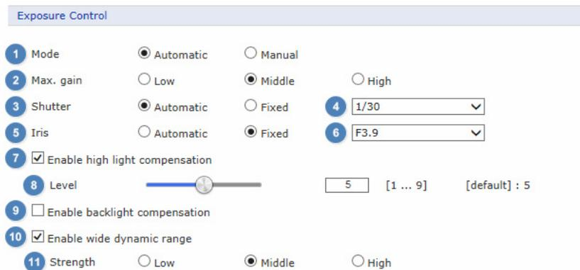
1. **Mode:** Determines exposure mode between automatic and manual. For automatic mode, at least one of Shutter and Iris should be set to automatic. For manual mode, both Shutter and Iris become fixed.
