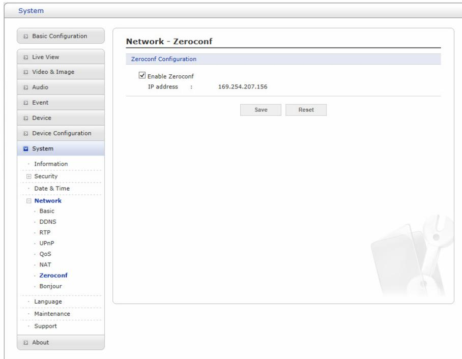
Zero configuration networking (zeroconf) is a set of techniques that automatically creates a usable Internet Protocol (IP) network without manual operator intervention or special configuration servers.
