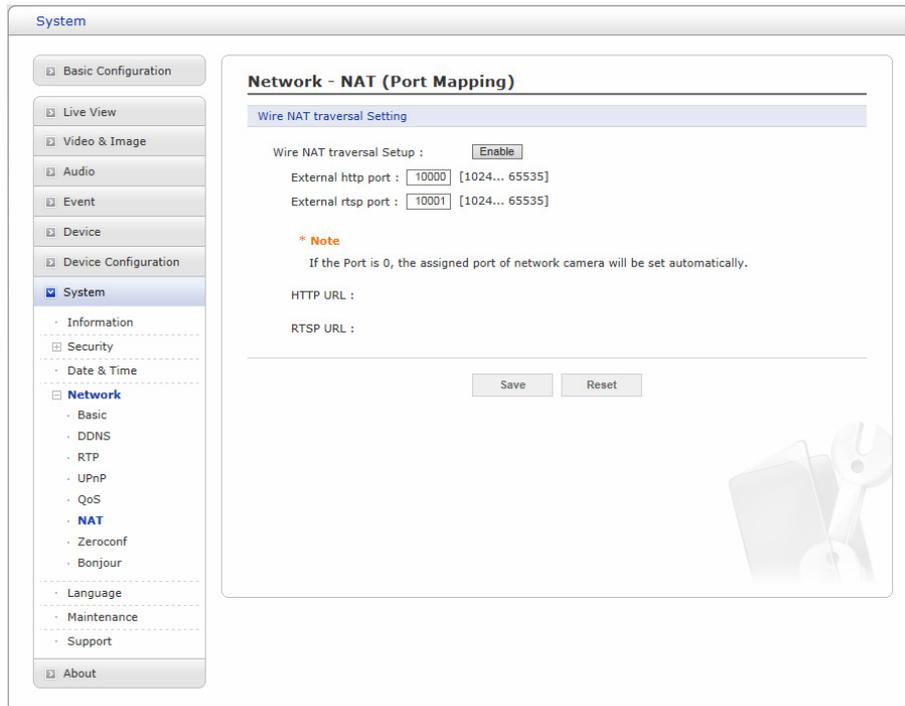
A broadband router allows devices on a private network (LAN) to share a single connection to the Internet. This is done by forwarding network traffic from the private network to the outside, that is, the Internet. Security on the private network (LAN) is increased since most broadband routers are pre-configured to stop attempts to access the private network (LAN) from the public network/Internet.
