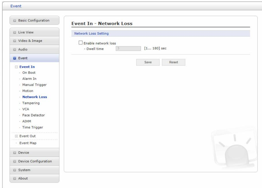
This is used to trigger an event every time the network connection is failed. Select “Enable network loss” to activate the Network Loss event. Select a dwell time for how long the event will last from the point of detection.
