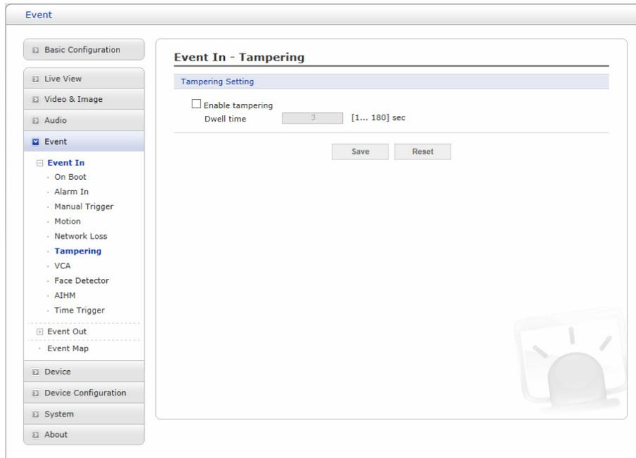
This is used to trigger an event when camera tampering occurs, for example, obstruct the camera with foreign material or move camera direction using external force. Select “Enable tampering” to activate the Tampering event.
