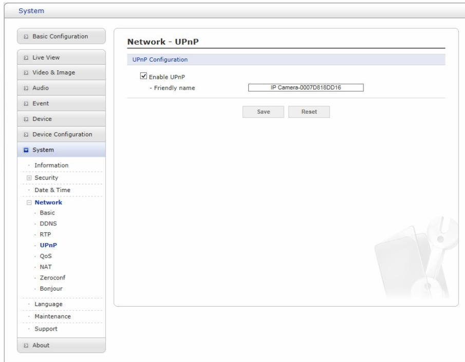
The network camera includes support for UPnP. UPnP is enabled by default, so the network camera is automatically detected by operating systems and clients that support this protocol.
