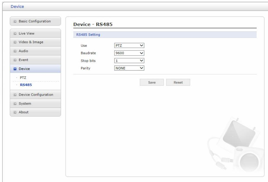
The screenshot displays a web-based configuration interface for a camera. The main content area is titled "Device - RS485" and contains a section for "RS485 Setting". This section includes four dropdown menus: "Use" set to "PTZ", "Baudrate" set to "9600", "Stop bits" set to "1", and "Parity" set to "NONE". Below these settings are two buttons: "Save" and "Reset". The left sidebar shows a navigation menu with "Device" selected and expanded to show "PTZ" and "RS485".
