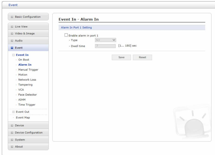
This camera provides Alarm In ports and user can set each ports individually. Each Port can be given as Normally Open or Normally Close state, and their Normal state can be configured. In order to use an alarm port, check the desired “Enable alarm port #” first.
