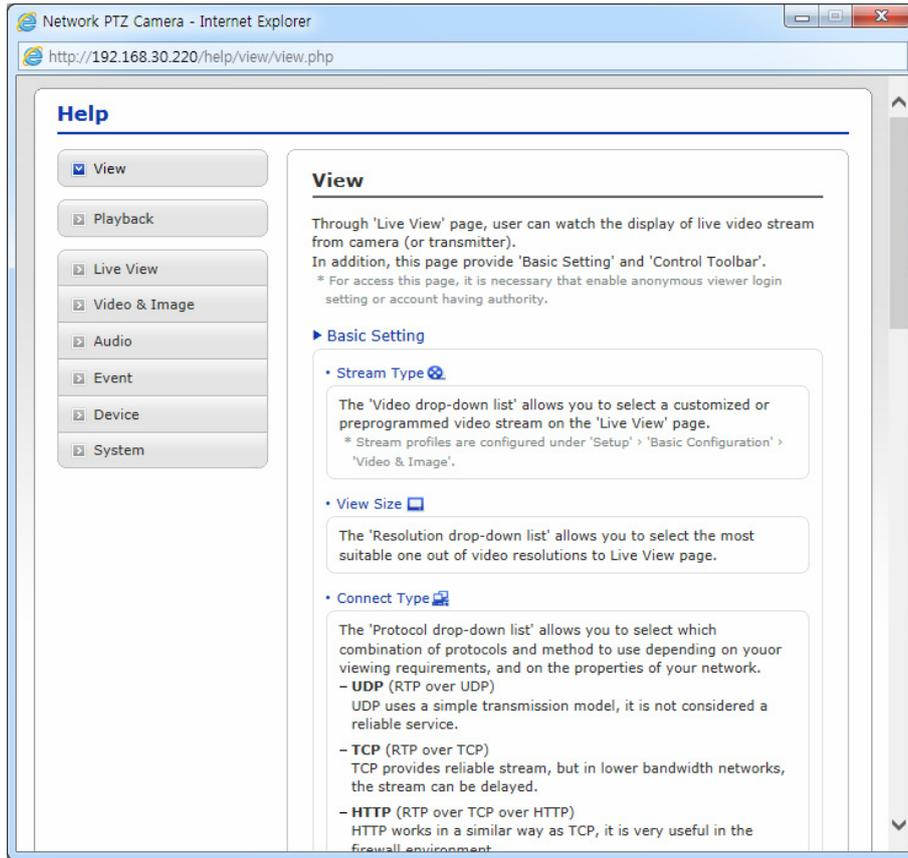
The Help information window will be provided as a popup window so that users can open and read it without needing to log-in. It will offer a description of the setting and Help page so that users can manipulate the network camera without a reference to the manual.
